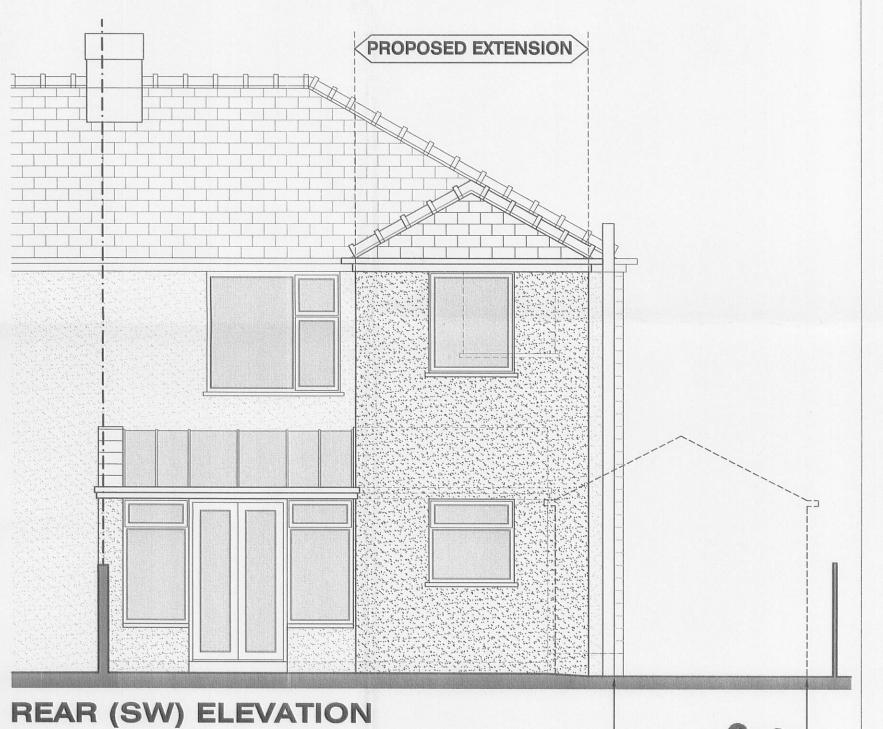
EXISTING SOIL VENT PIPE TO BE REPOSTIONED TO SUIT NEW EXTENSION -
