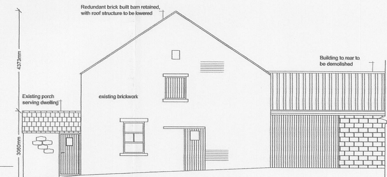
existing east facing elevation 1:100
