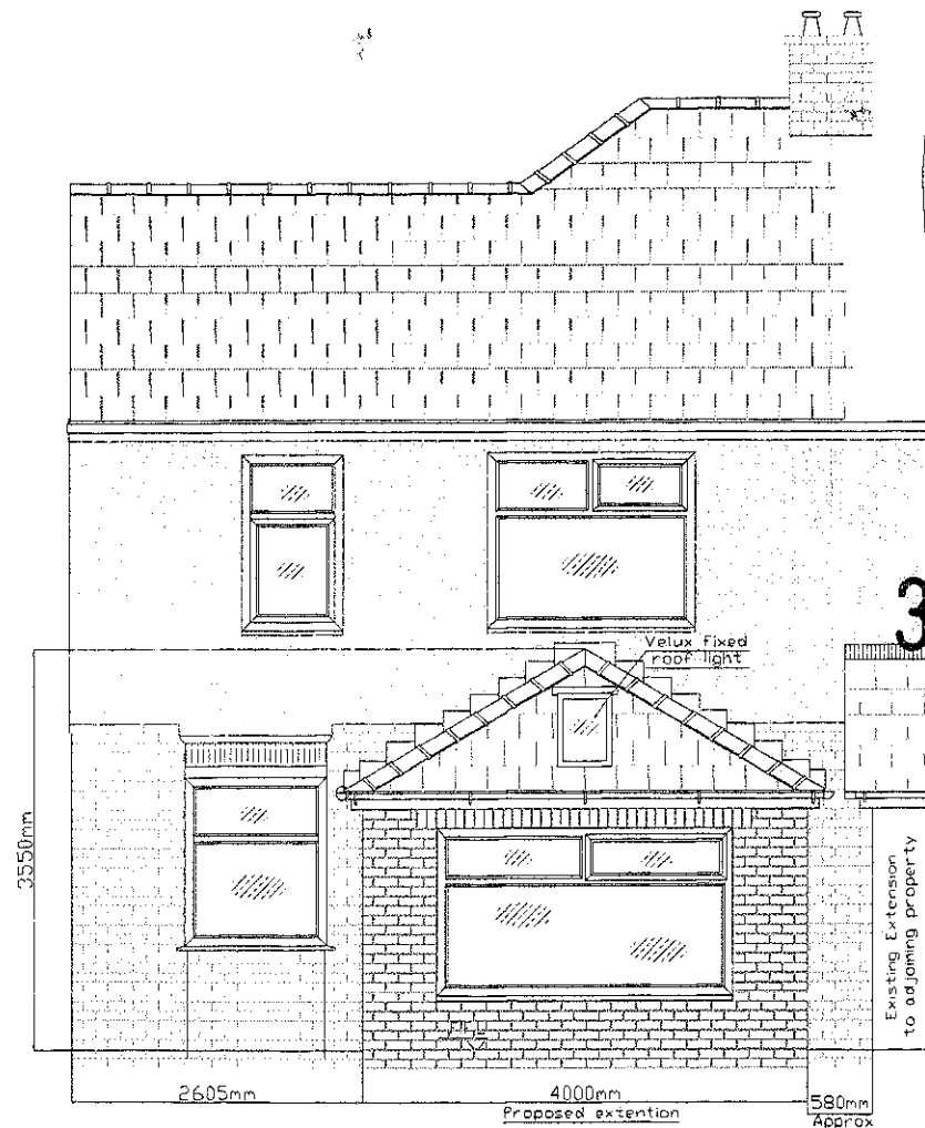
Proposed Rear Elevation Scale 1:75
