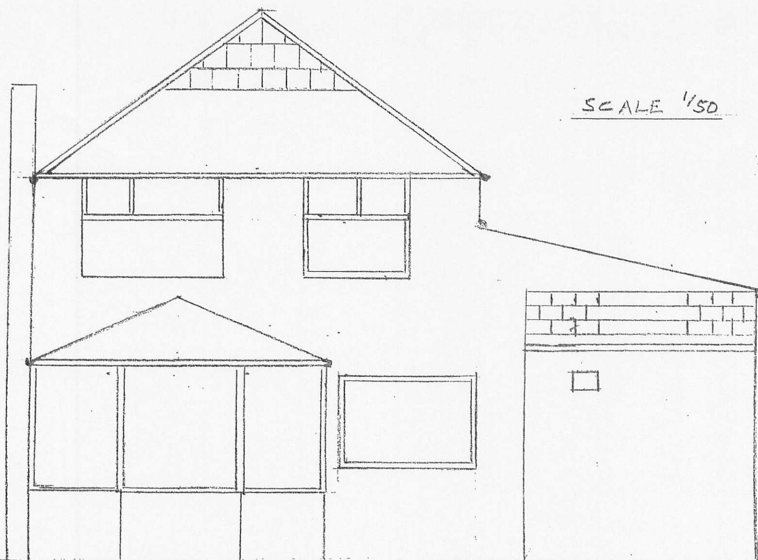
EXISTING REAR ELEVATION
