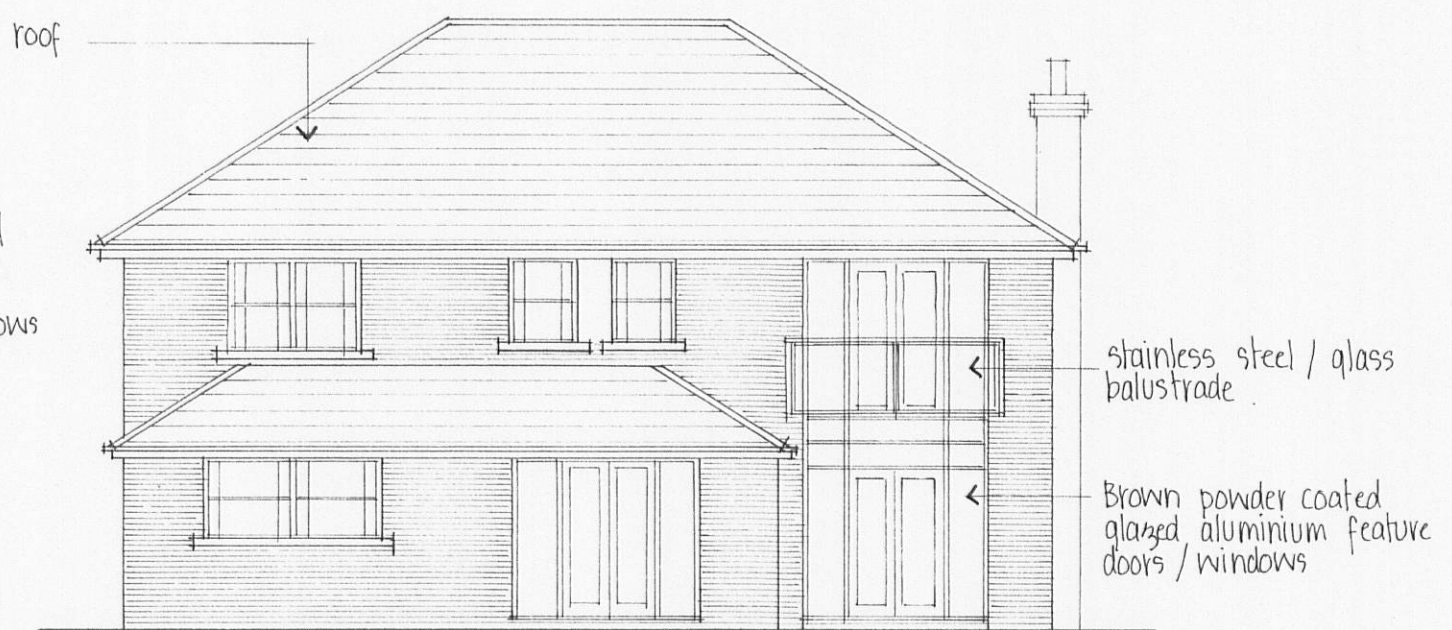
SOUTH WEST ELEVATION
