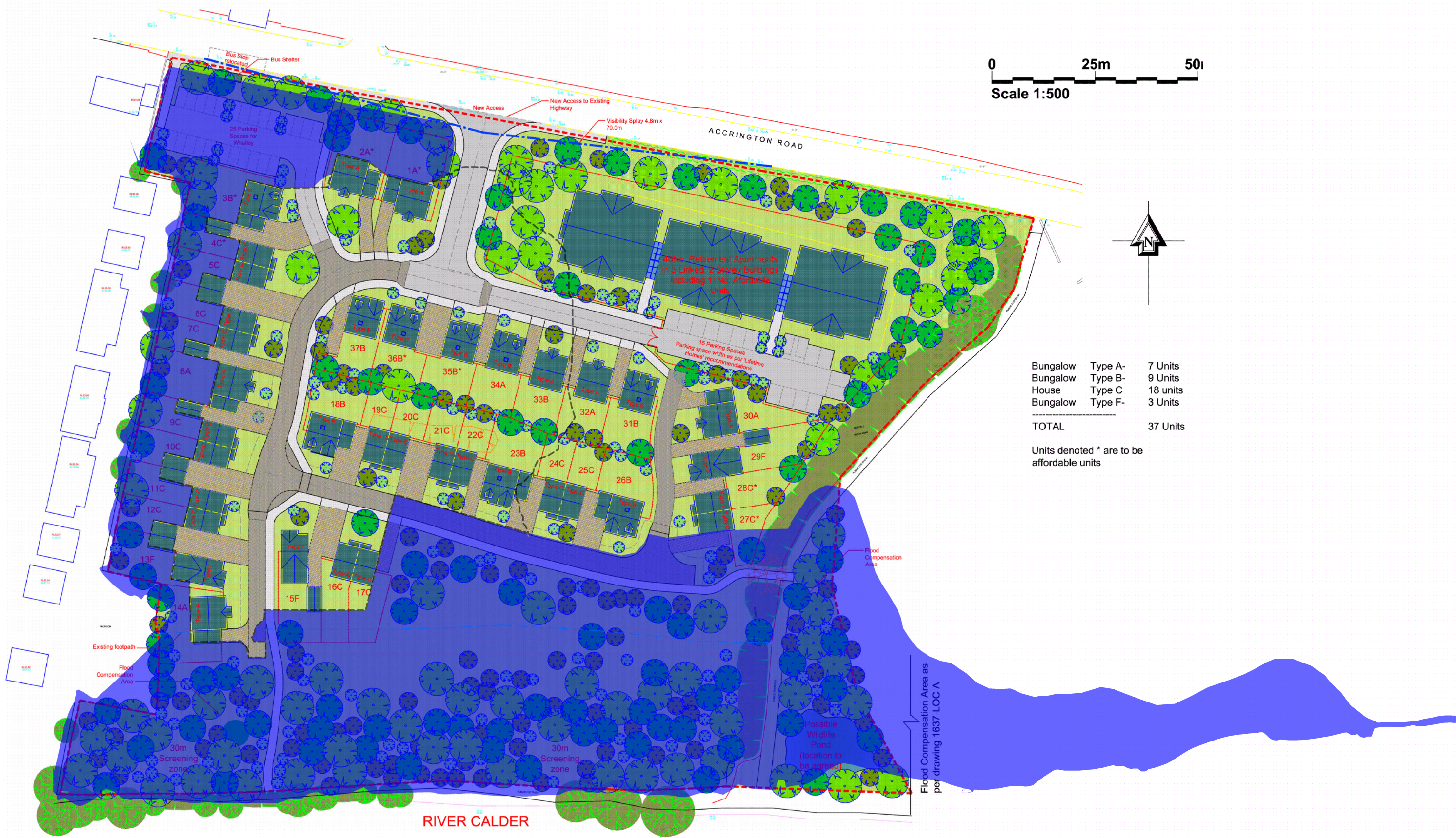
Figure 6: Maximum flood extent under the design event overlaid onto the proposed development scheme.
