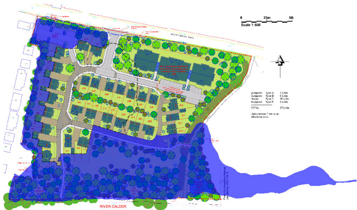
Figure 7b: Schematic: Maximum flood extent under the design event overlaid onto the proposed development scheme.
