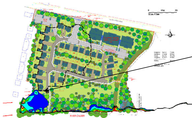
Figure 3: Delineating the 45.7m AODN contour. Floodwater is prevented from flowing further northwards due to a naturally high section of ground.
