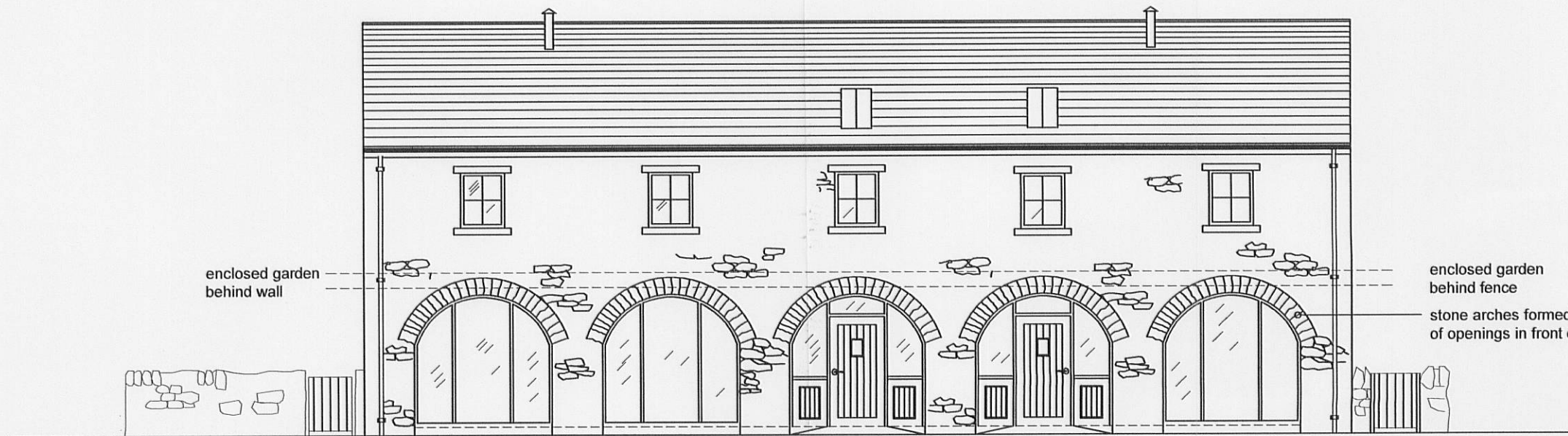
South West Facing Elevation 1:100
