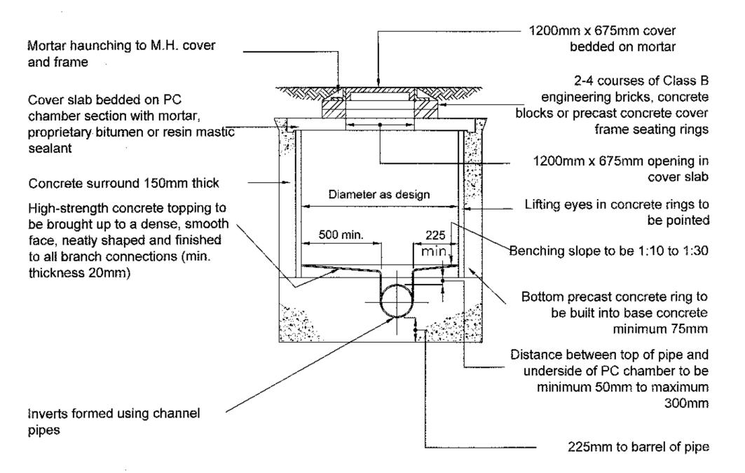
**TYPICAL MANHOLE DETAIL-TYPE 4** depth to soffit 1.0m to 1.5m
