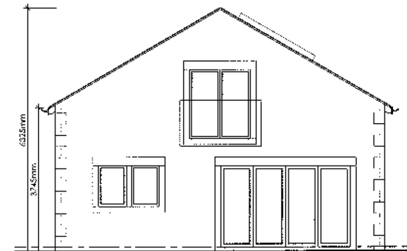
South West Elevation 1:100
