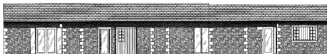
Cottage Three and Four (Front elevations) some alterations to allow for new door openings
