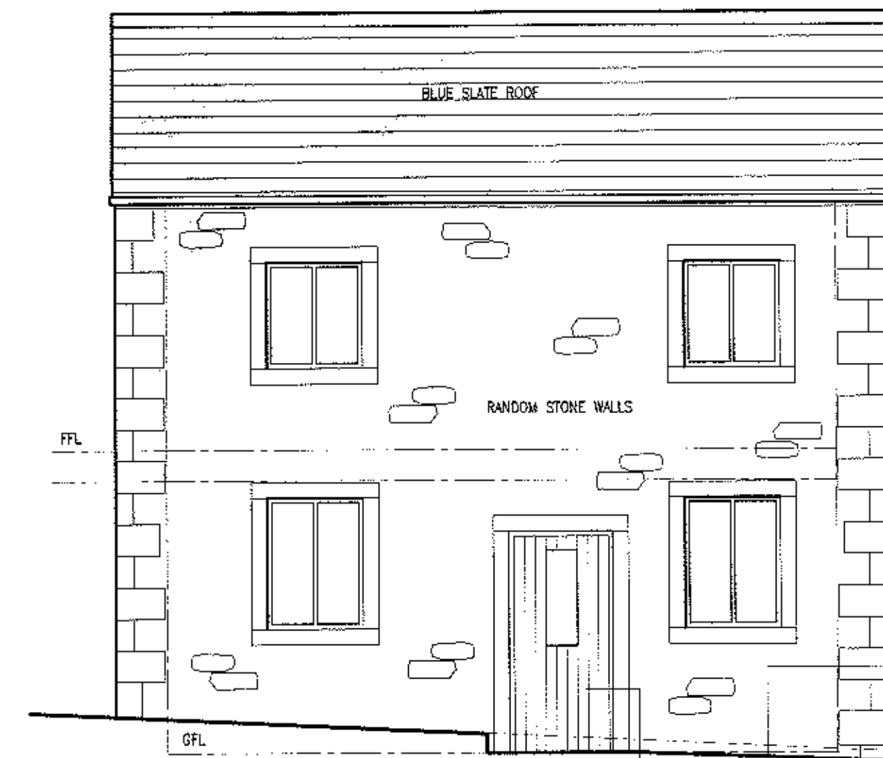
NORTH WEST ELEVATION
