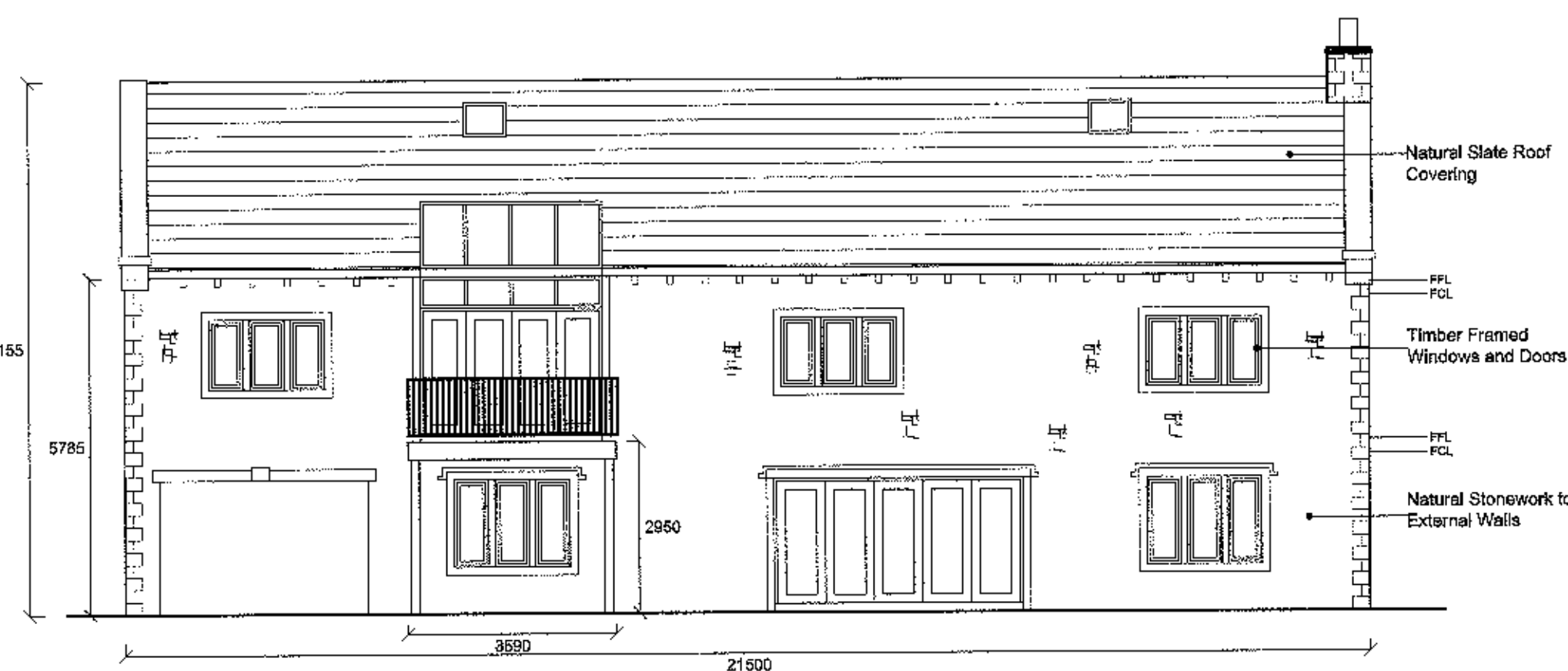
Rear (North) Elevation
