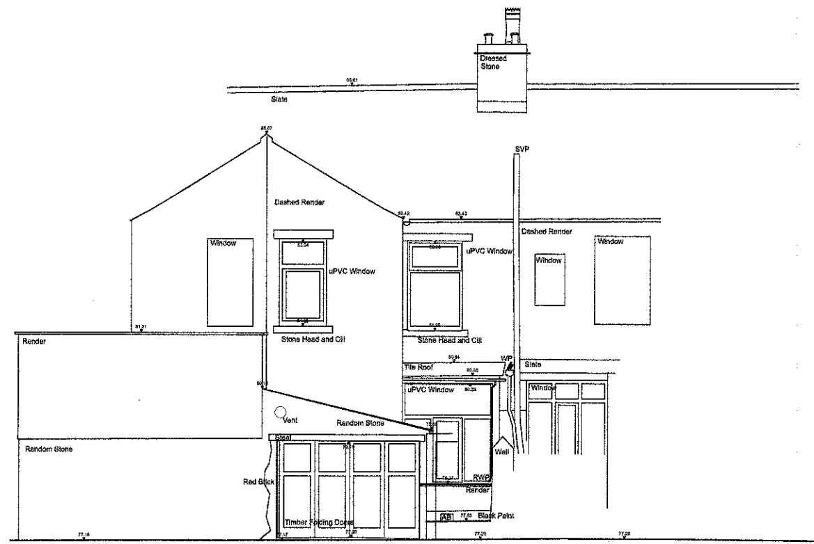
existing east elevation
