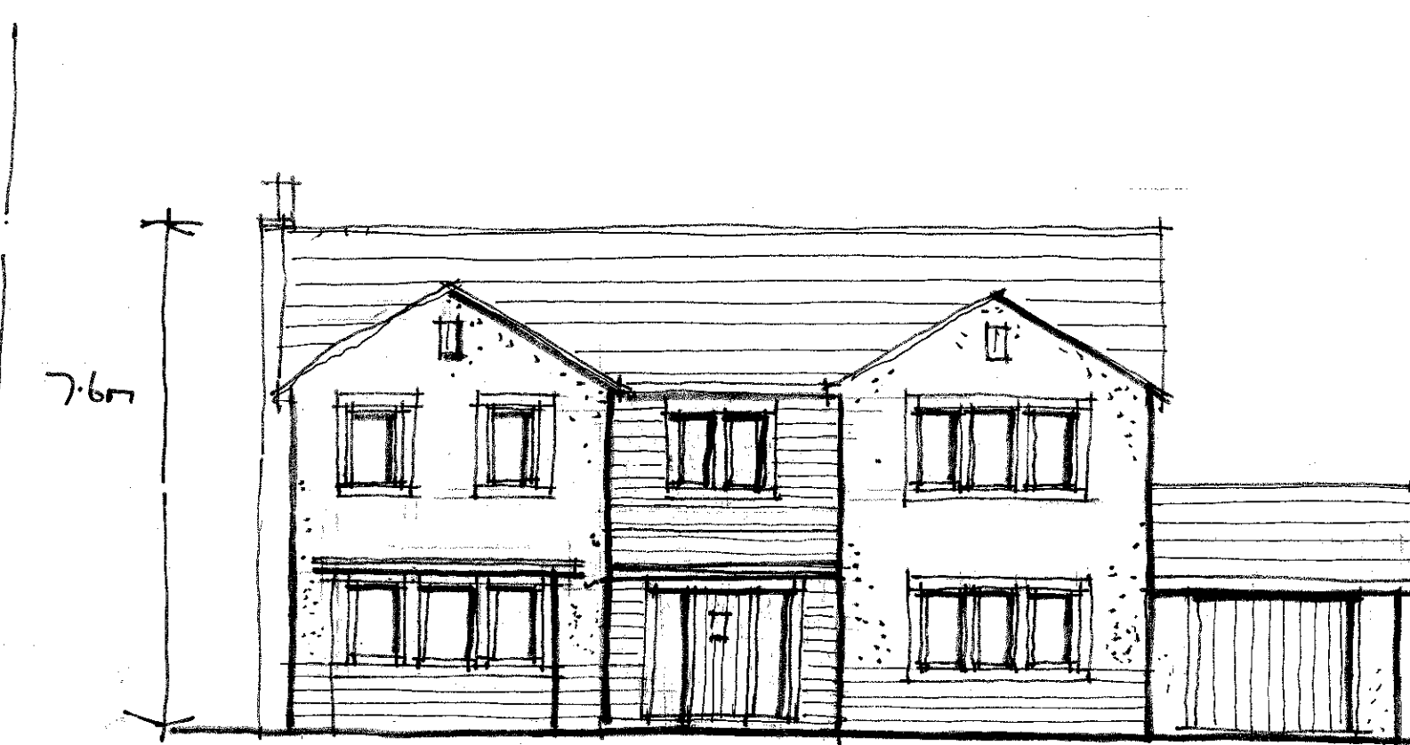
NORTH WEST ELEVATION 1:100
