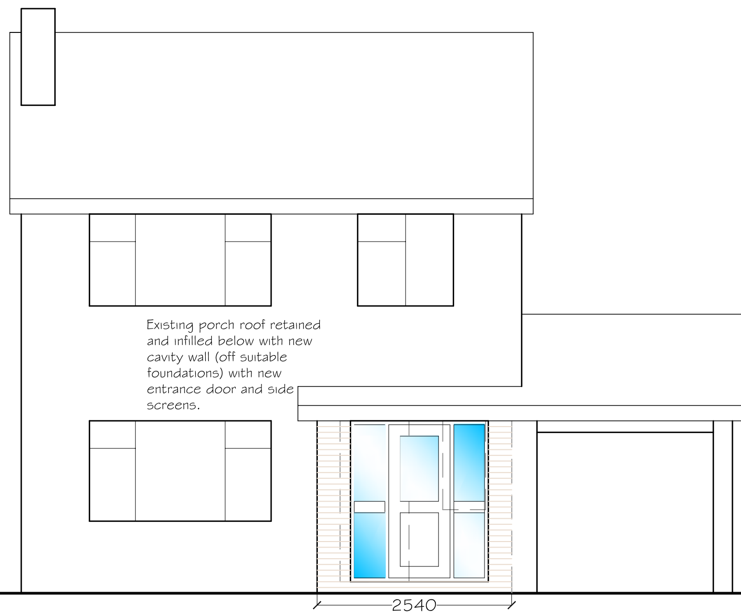
FRONT ELEVATION North West
