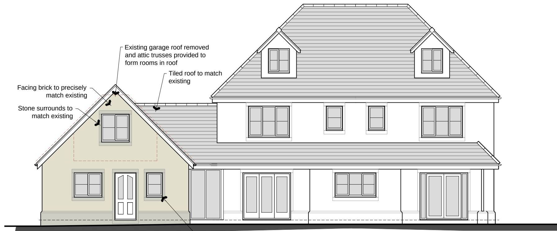
South West Elevation
