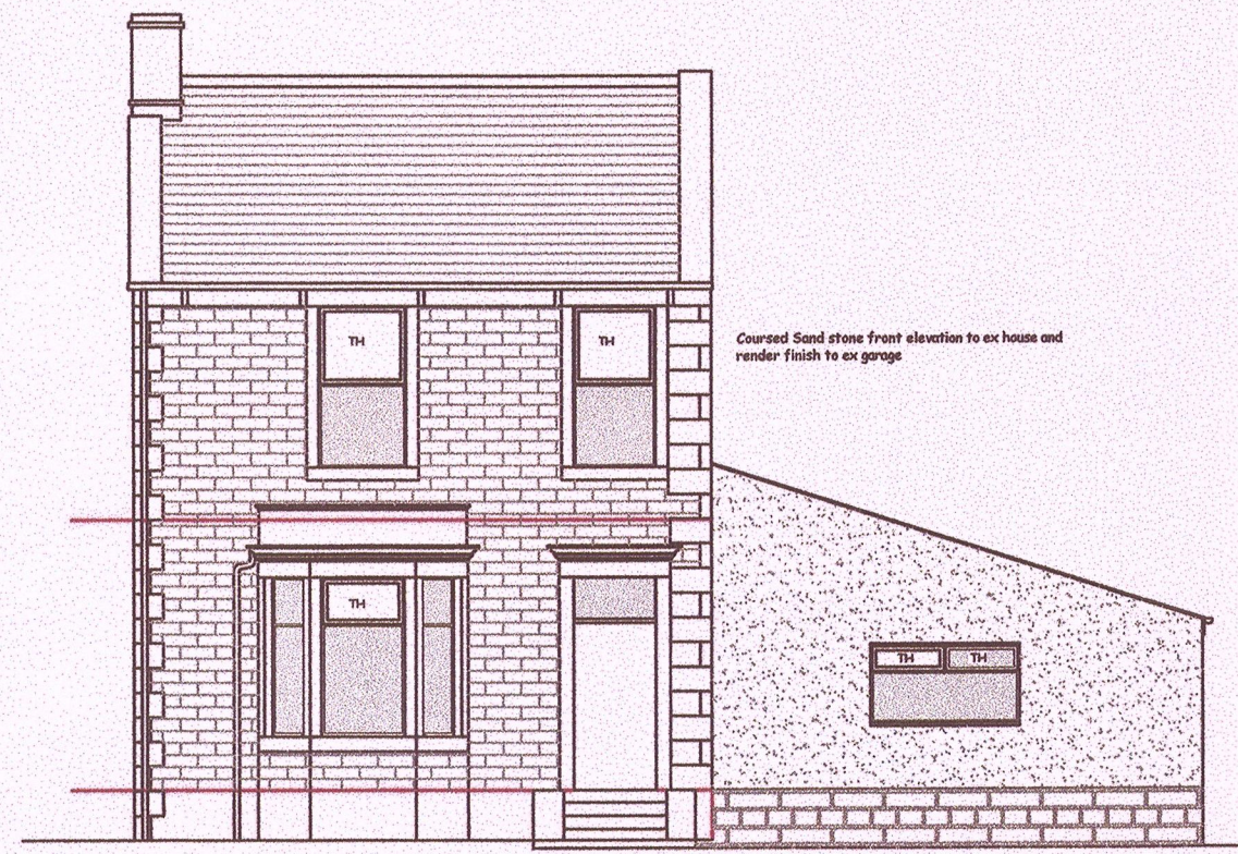
Existing Front Elevation
