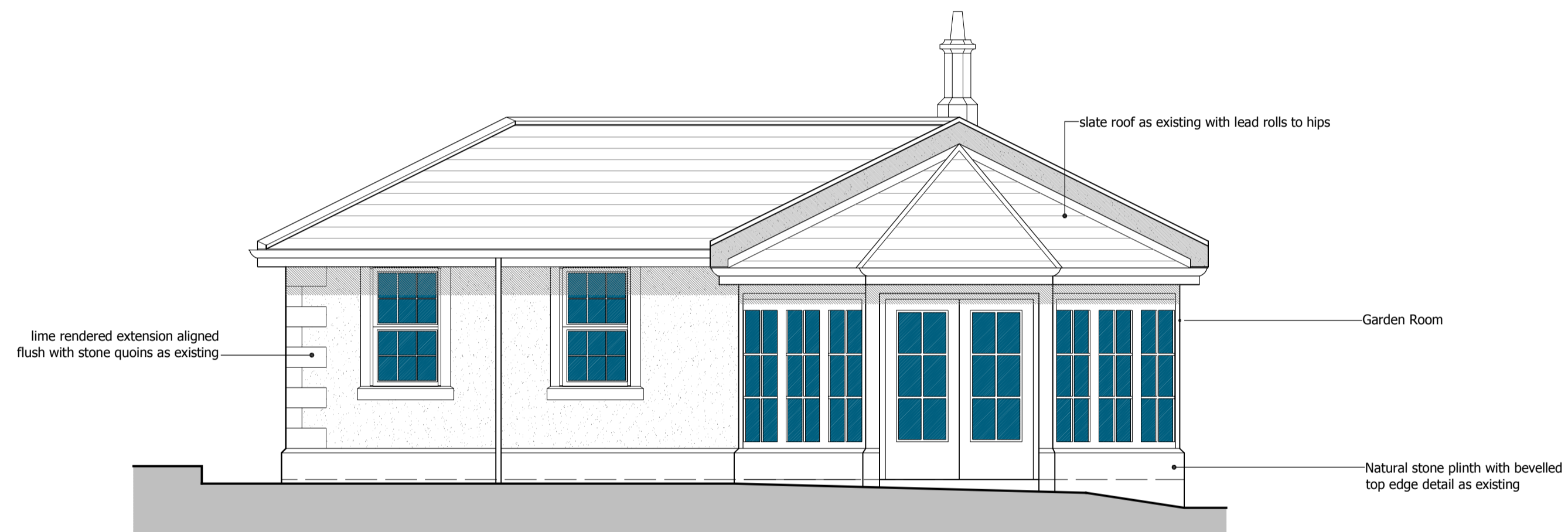
SOUTH WEST ELEVATION
