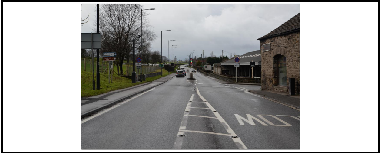
Approach from east side showing refuge and ghost island preventing overtaking
