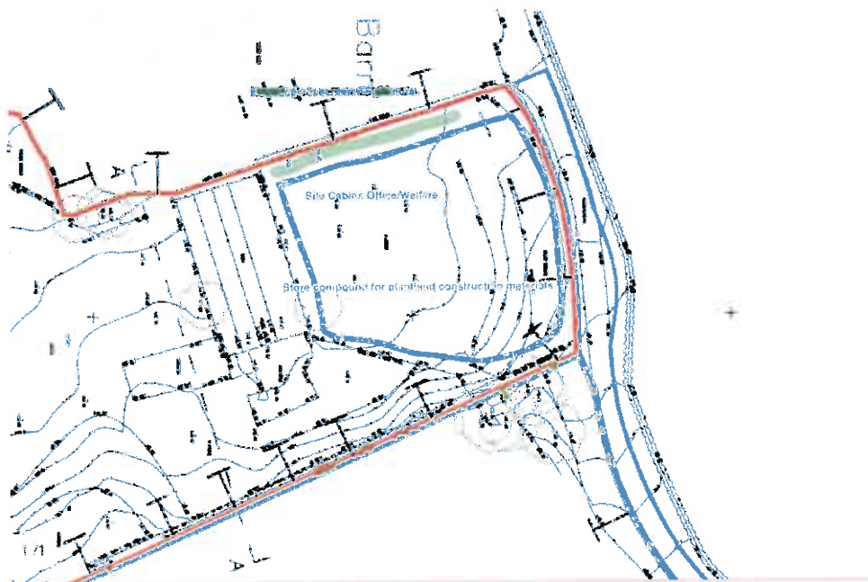
Compound for Plant machines, Site Cabins and Material Storage (Wheel Washing)
