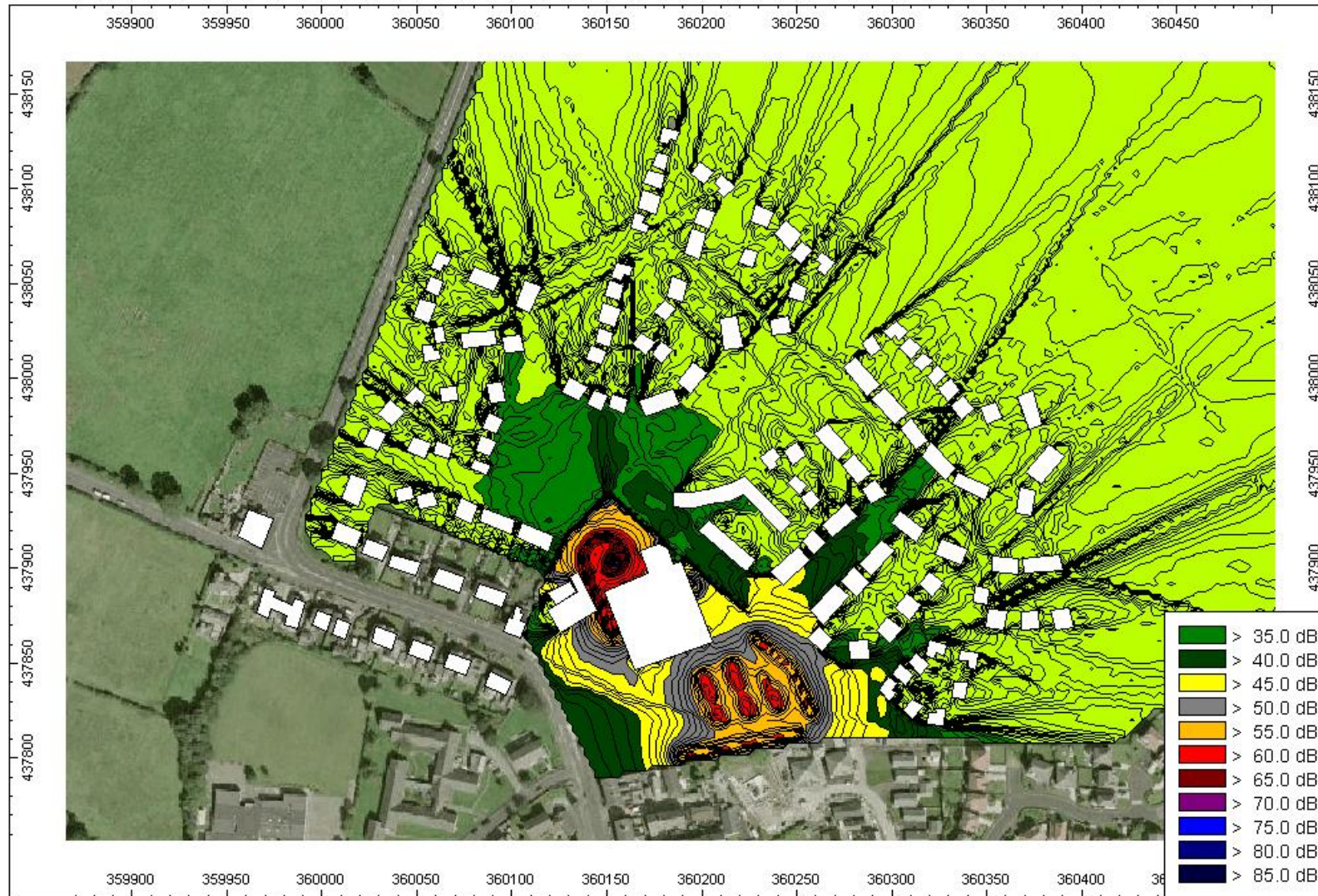
Figure D.3 – Modelled Ground Floor Daytime Noise Levels for Operational Activities Associated with Sainsbury's Supermarket With Mitigation Measures in Place (Figures in dB L_{Aeq, 1hour} )
