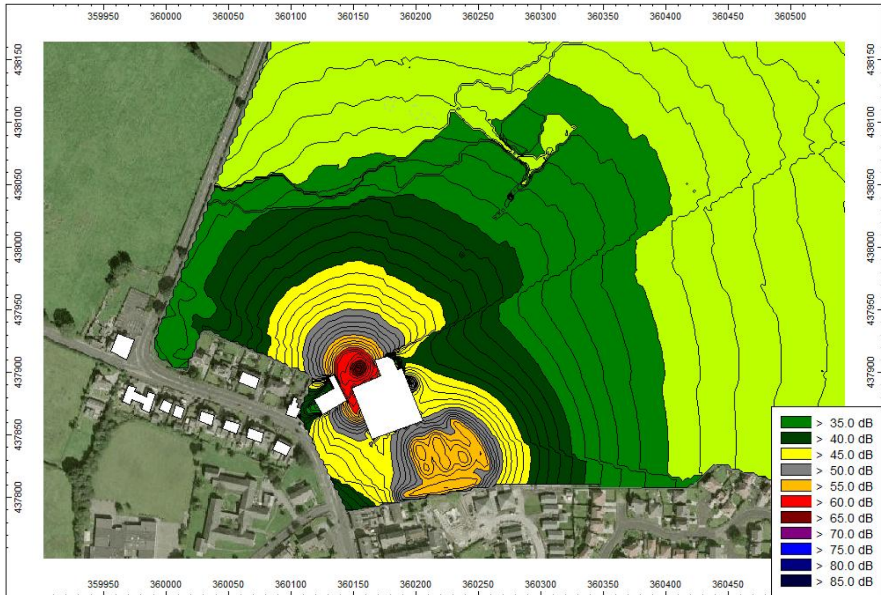
Figure D.2 – Modelled First Floor Night-time Noise Levels for Operational Activities Associated with Sainsbury's Supermarket Without Mitigation Measures in Place (Figures in dB L_{Aeq, 1hour} )
