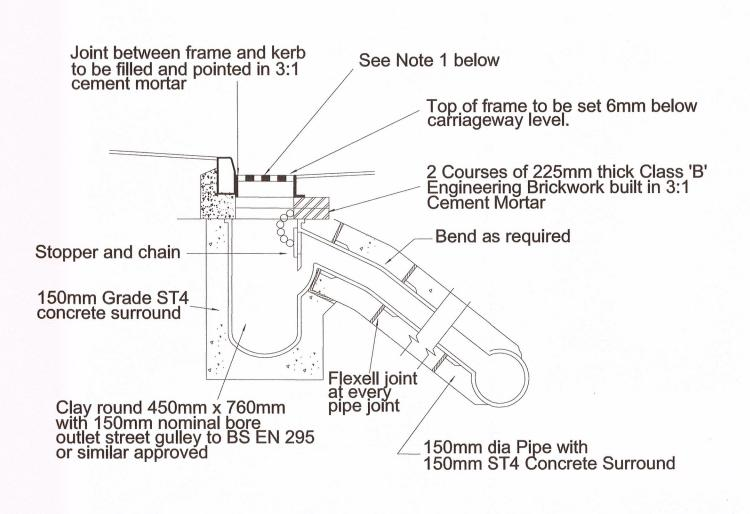
1. Gully grating and frame to BS EN 124 Class C400 to be of hinged, rectangular, (Approved Tester Kite mark or LRQA) Set in 3:1 Cement Mortar
