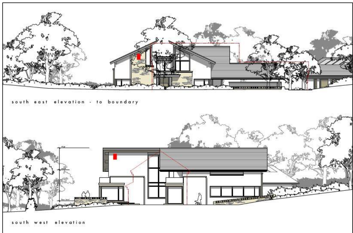
Plate 25: Locations of the new Schwegler 1FR bat boxes (red) to be built into the structure of the new building.
