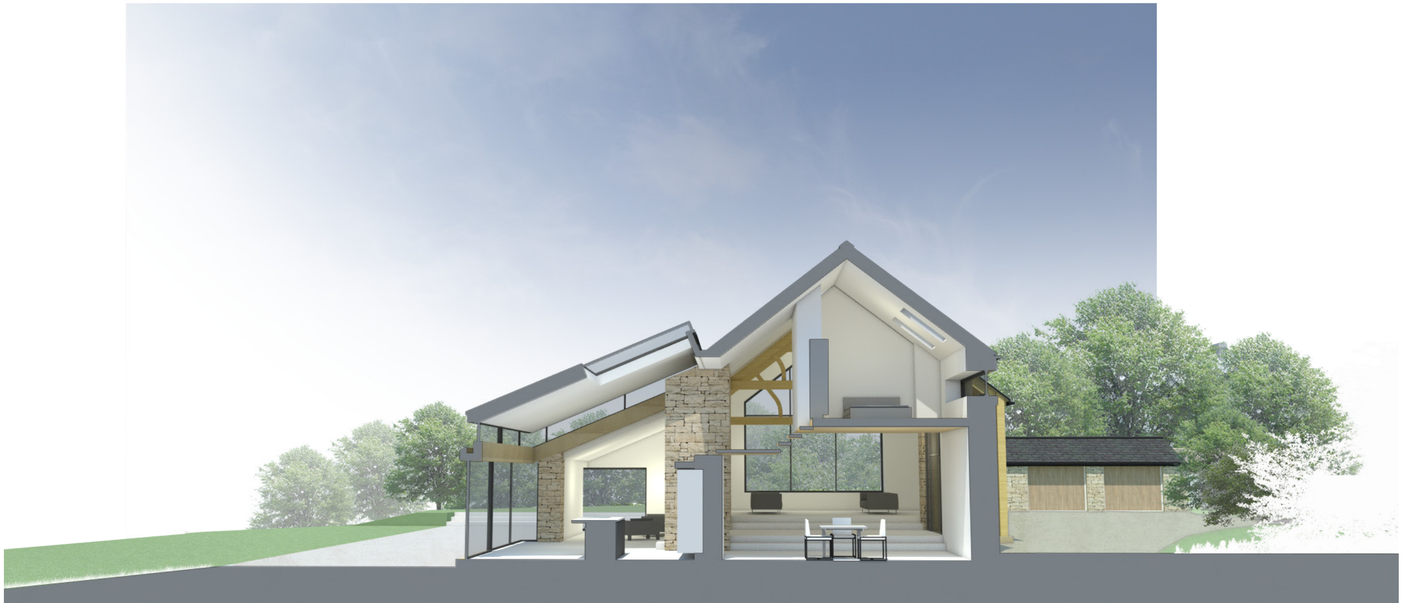
Section through barn and extension
