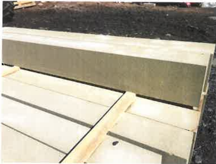
Pl. 3 Photograph showing natural buff coloured sandstone for the proposed extension jambs and cills
