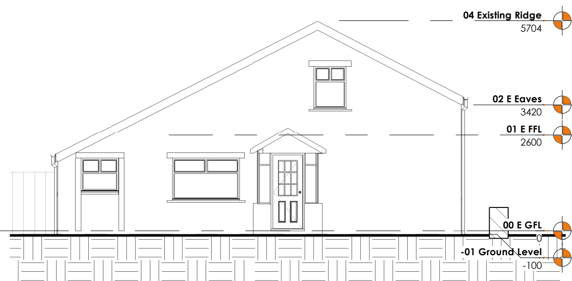
E2 Existing /side (west) Elevation 1 : 100 N188
