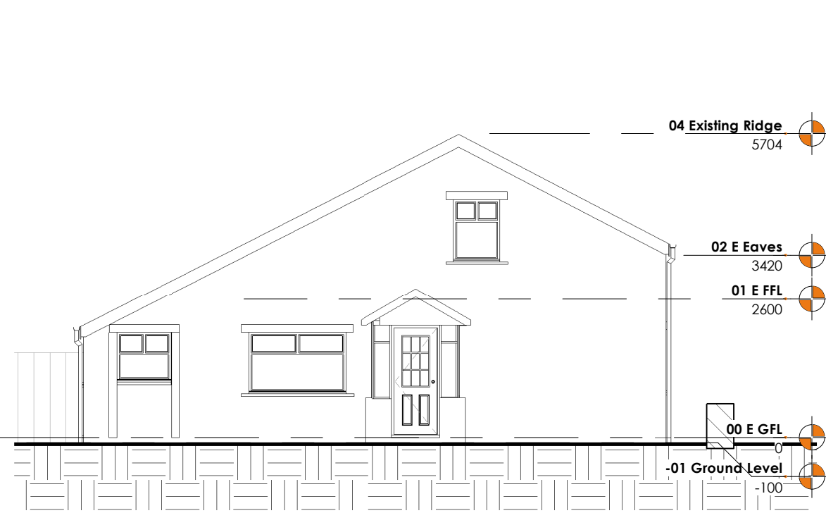
E2 Existing /side (west) Elevation 1 : 100 N188
