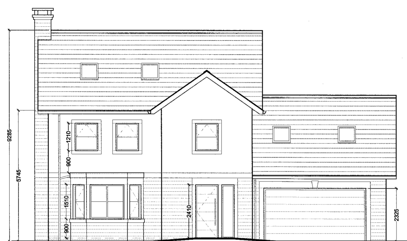
South West (Front) Elevation 1:100 Scale
