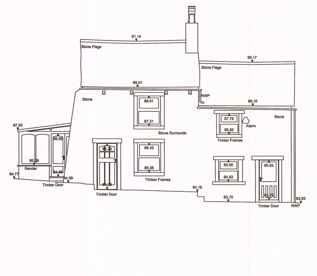
South Elevation ▼ 80.00m above OS Datum
