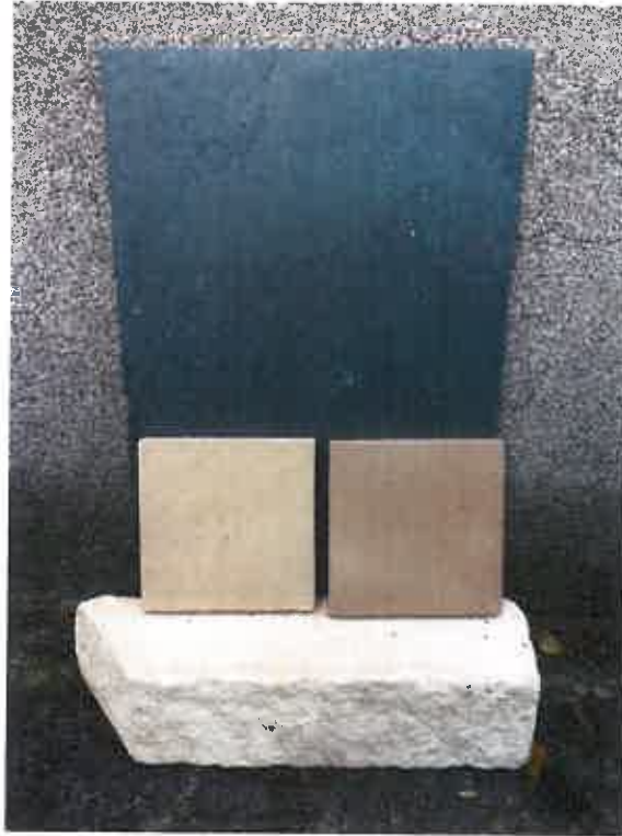
Pl. 1 Photograph showing buff textured natural stone for all external walls which would be laid to random coursed varying from 65, 90, 115 and 140mm courses (no quoins), below samples of dressed natural buff stone for all window / door surrounds, string coursing and chimney cap detailing. It also shows how this would appear next to the proposed natural blue slate (Spanish) for all pitched roofs (shown behind the stone).
