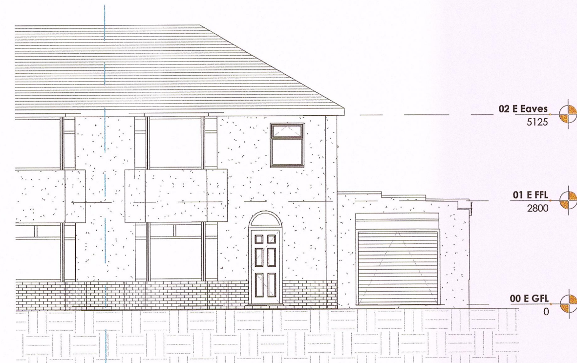
E1 Existing Front (west) Elevation 1 : 100 N160
