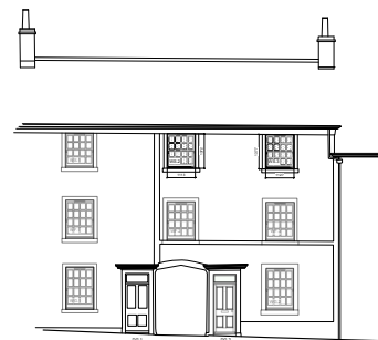
Proposed South East Elevation - Proposed Replacement of Windows WS.2 and WS.3
