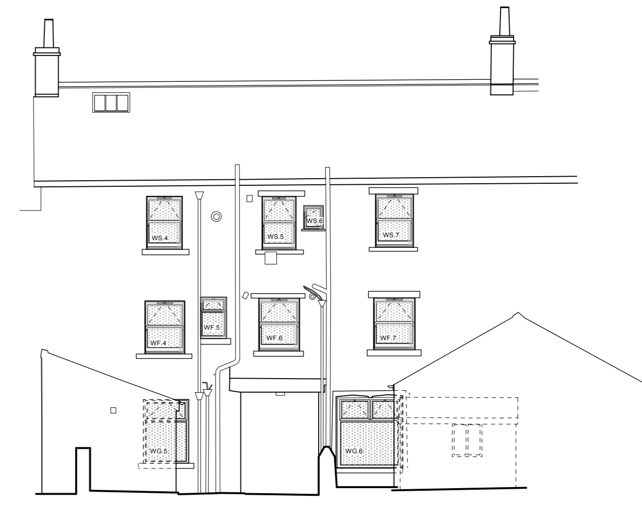
Proposed North West Elevation - Proposed Replacement of Windows to Rear Elevation, as Details Below. 1:100
