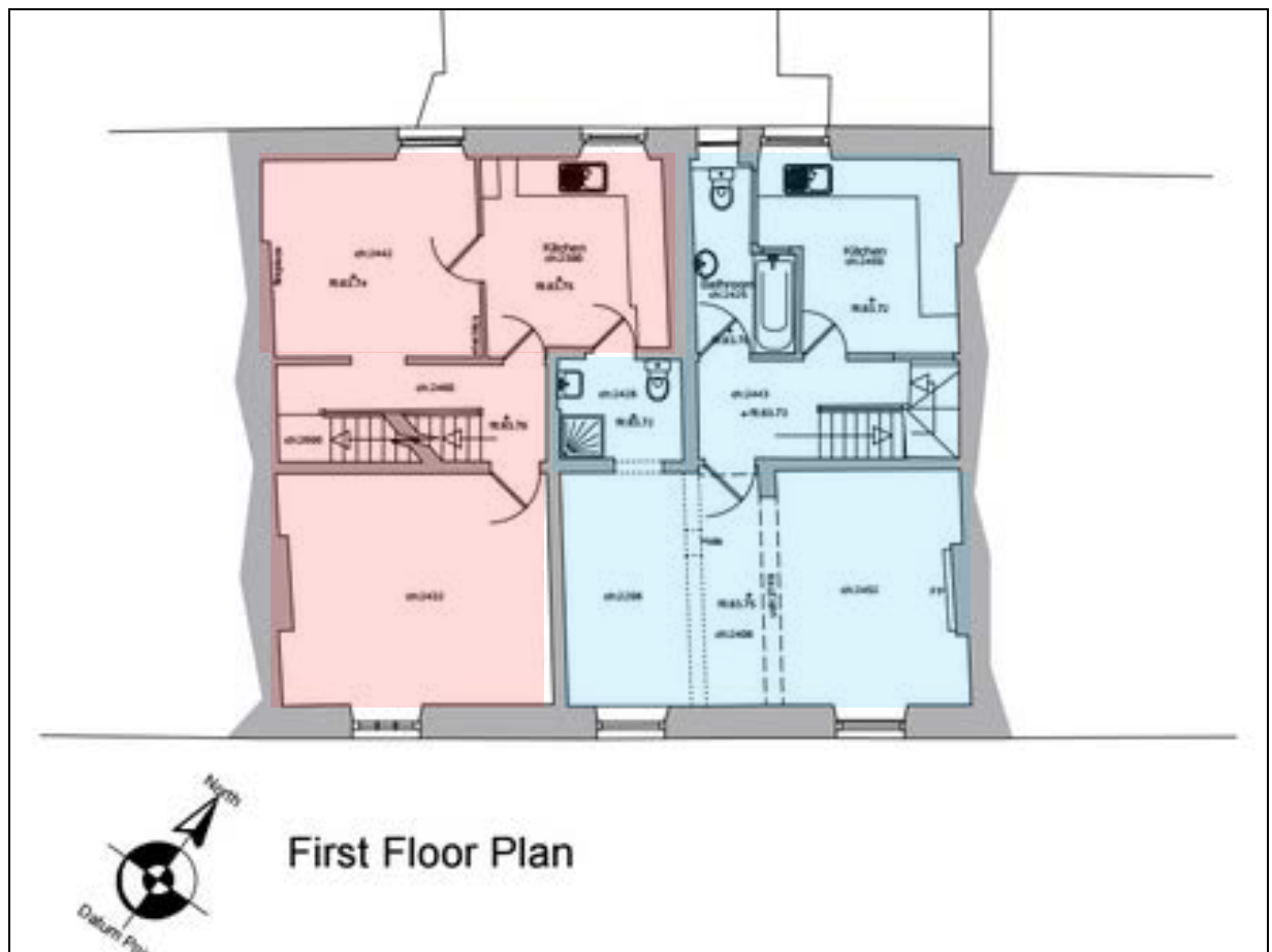
12. Present first floor plans: shading indicates original extent of each house (IWA Architects Ltd)
