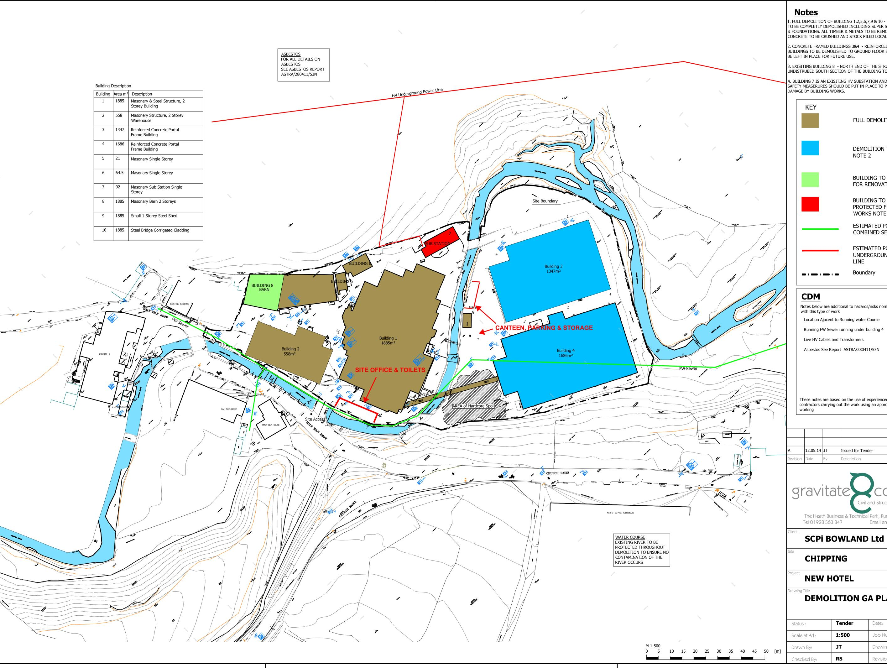
. FULL DEMOLITION OF BUILDING 1,2,5,6,7,9 & 10 - EXISTING BUILDING STRUCTURE TO BE COMPLETLY DEMOLISHED INCLUDING SUPER STRUCTURE, GROUND FLOOR SLAE & FOUNDATIONS. ALL TIMBER & METALS TO BE REMOVED OFF SITE. MASONARY & CONCRETE TO BE CRUSHED AND STOCK PILED LOCALLY. REBAR TO BE REMOVED.
