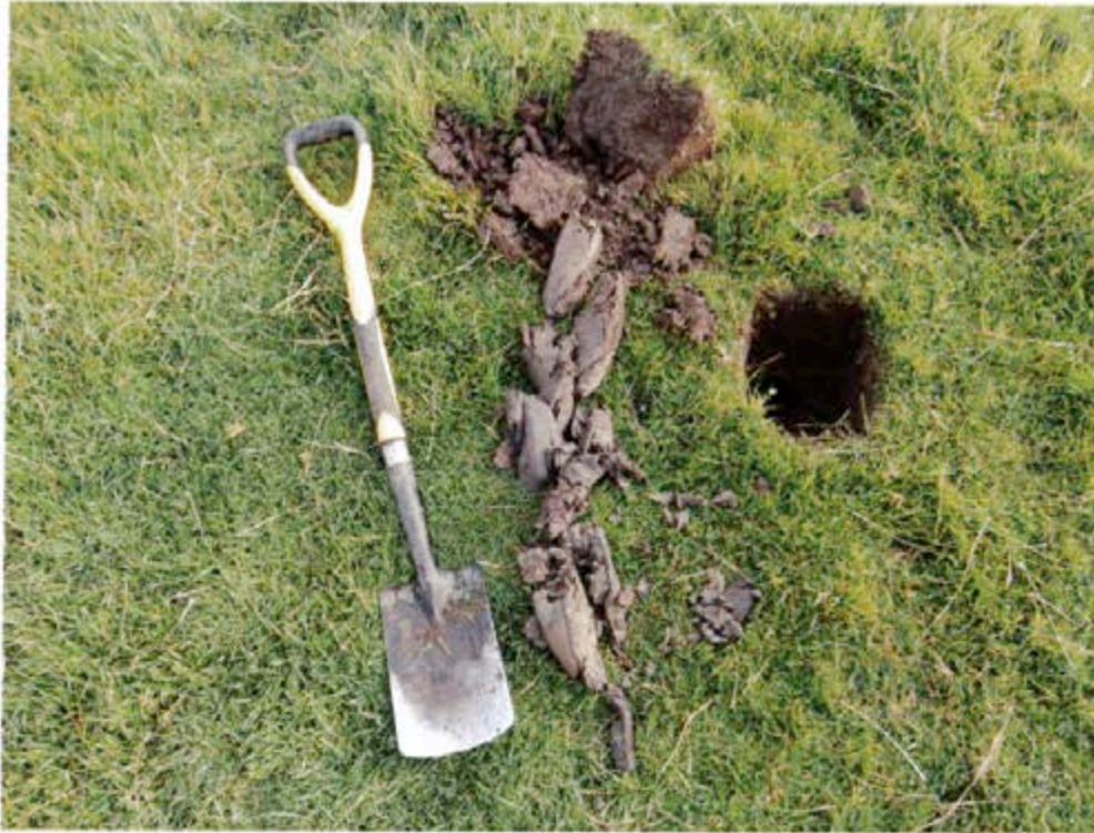
Fig (v) : Typical soil profile – 200mm loam overlying clay.
