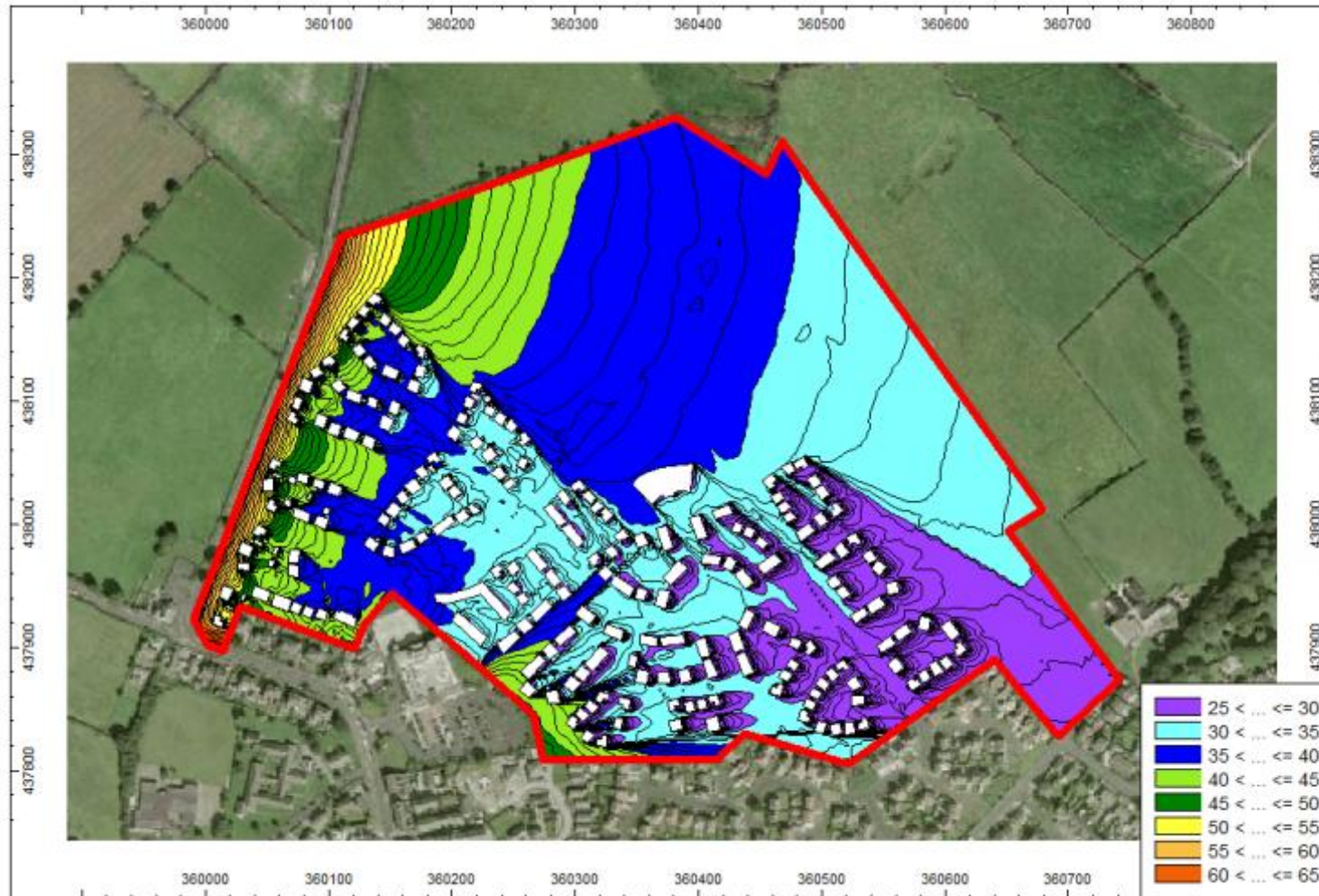
Figure E.1 – Modelled Ground Floor Daytime Road Traffic Noise Levels With the Development in Place (Figures in dB L_{Aeq, 16} -hour)
