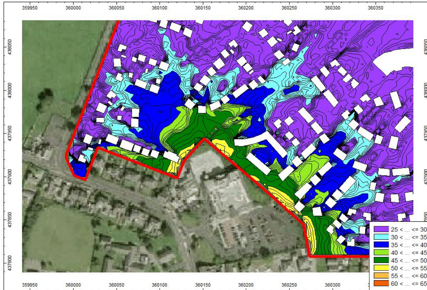
Figure E.4 – Modelled Ground Floor Daytime Noise Levels for Operational Activities Associated With Sainsbury's Supermarket, Ireland's Garage and Wash and Dash Car Wash, Without Mitigation Measures in Place (Figures in dB L_{Aeq, 1hour} )
