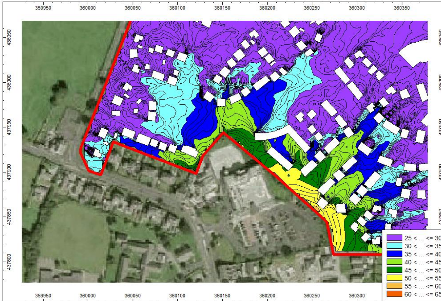
Figure E.6 – Modelled First Floor Night-time Noise Levels for Operational Activities Associated with Sainsbury's Supermarket With Mitigation Measures in Place (Figures in dB LAeq, 15-minutes)
