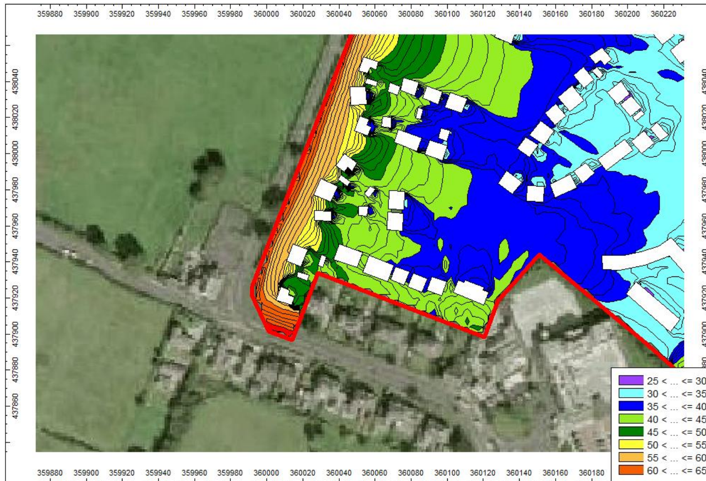
Figure E.3 – Modelled Ground Floor Daytime Road Traffic Noise Levels With Development and Mitigation Measures in Place (Figures in dB L_{Aeq, 16\text{-hour}} )
