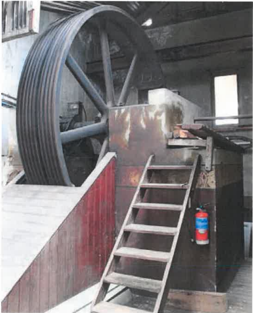
Plate 103: Substantial bed for secondary motion shaft housing
