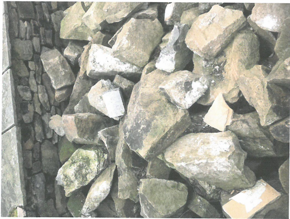
PLATE 8 IMPORTED RANDOM LOCAL SAND STONE FOR BUILDING WORKS SELECTED USED TO BUILD MATCHING WALLING INTO NEW SUN LOUNGE WALLS
