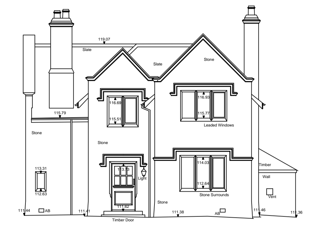
East Elevation ▼ 110.00m above OS Datum
