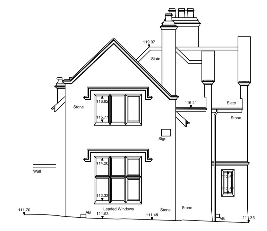
South Elevation ▼ 110.00m above OS Datum
