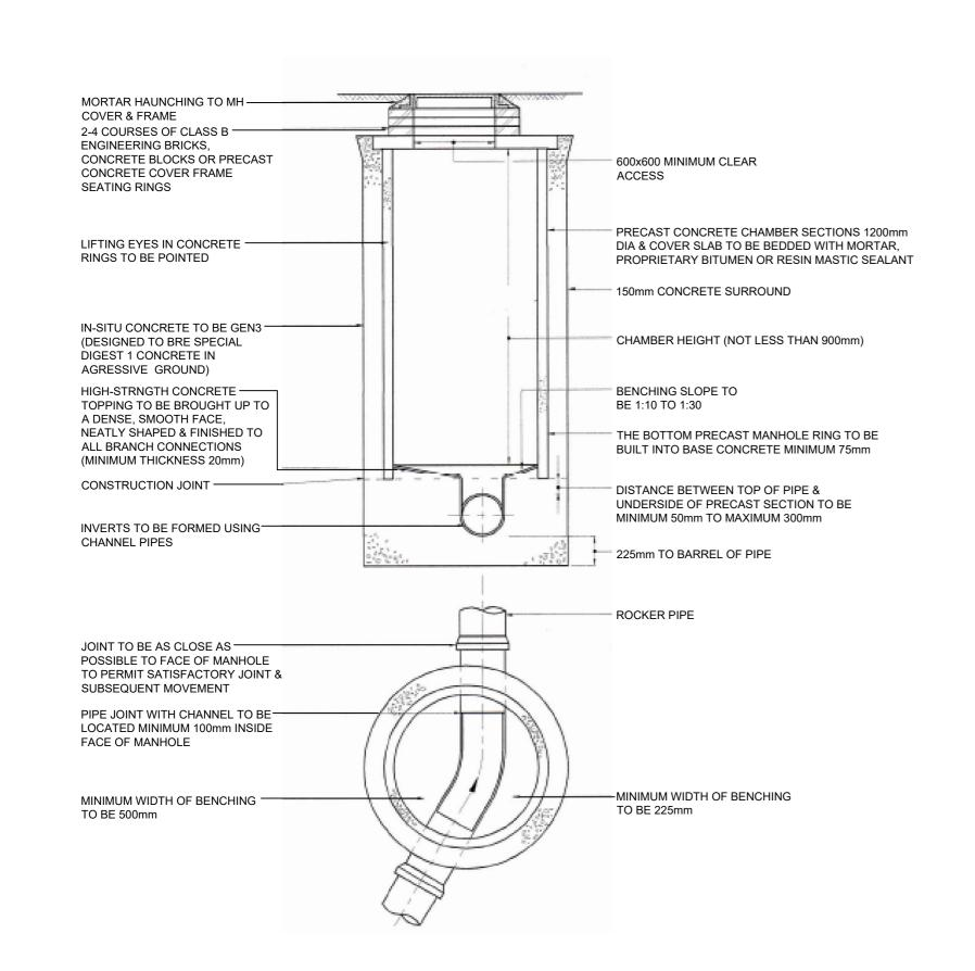
TYPICAL MANHOLE DETAIL - TYPE B
