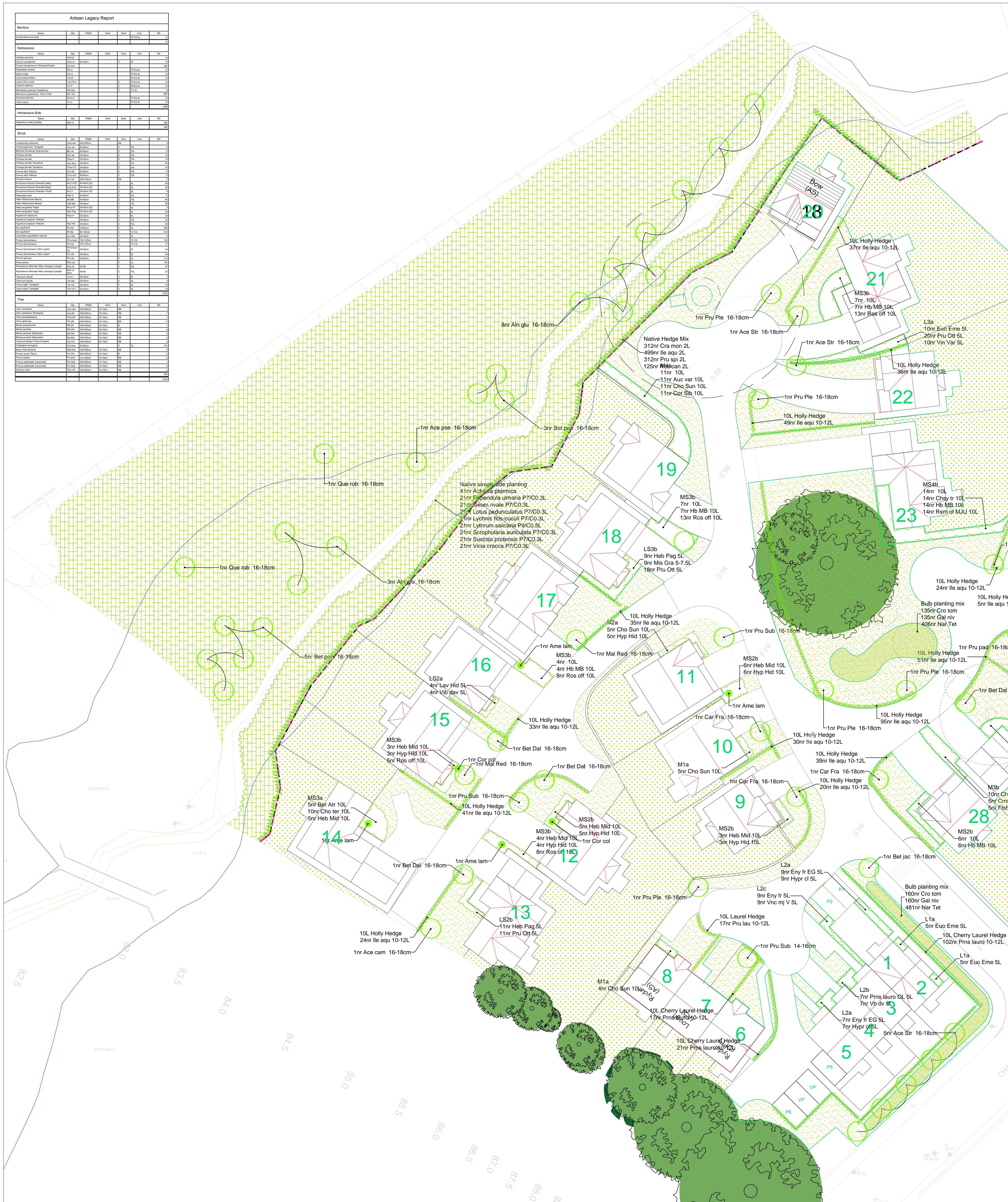
Extra heavy standard tree planting in grassed or planted areas. Tree pits to measure a minimum of 900mm x 900mm x 750mm deep, and at least 600mm wider than the root spread. To include single 1.6m timber stake, 600mm above ground, spacer tie.
