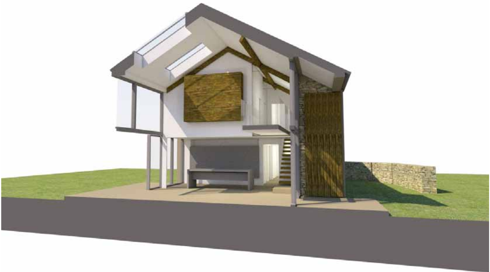
Section showing the double height space between waggon doors and new window, with bridge link across
