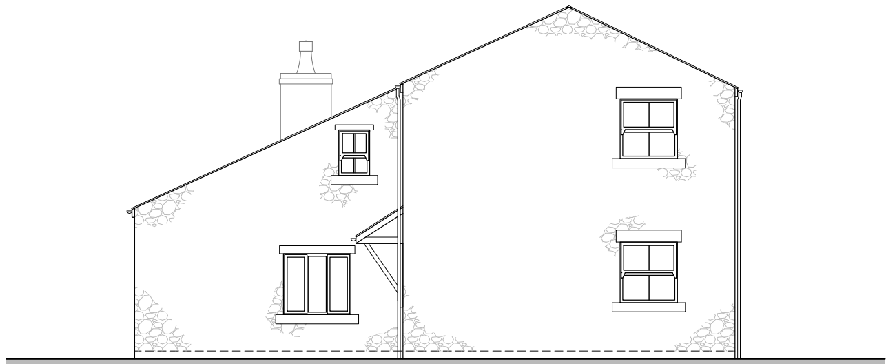
Existing Front Elevation (1:100)
