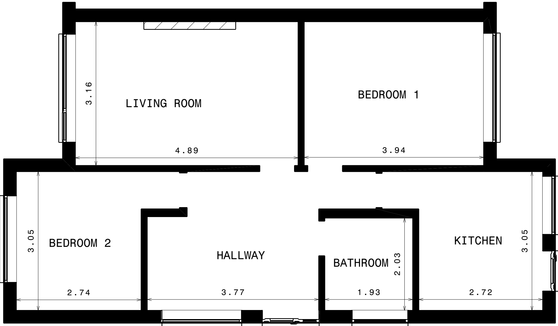
GROUND FLOOR - EXISTING Scale: 1:50
