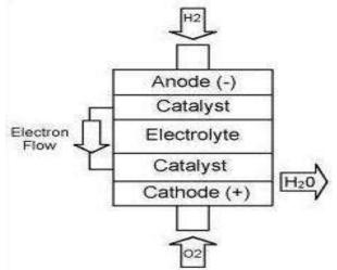
Hydrogen fuel is fed into the "anode" of the fuel cell. Oxygen (or air) enters the fuel cell through the cathode. Encouraged by a catalyst, the hydrogen atom splits into a proton and an electron, which take different paths to the cathode. The proton passes through the electrolyte. The electrons create a separate current that can be utilized before they return to the cathode, to be reunited with the hydrogen and oxygen in a molecule of water.
