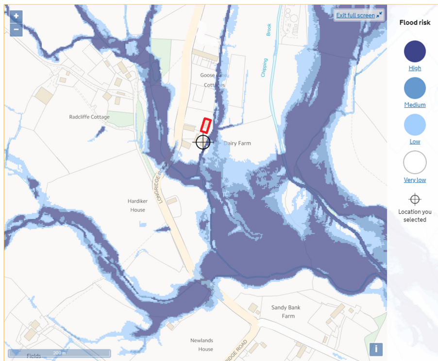
Figure 3 – Flood Risk from Surface Water
