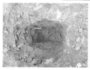
Plate 1: Trial Pit TP01 – Showing Made Ground
