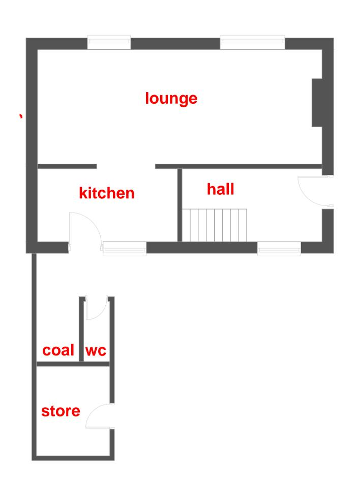
EXISTING GROUND FLOOR PLAN Scale 1:50
