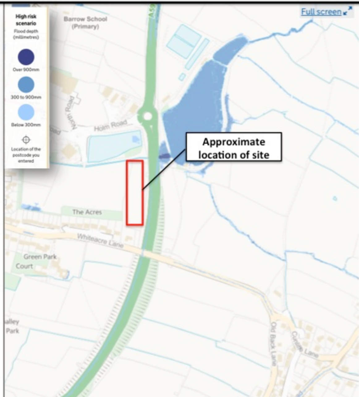
Figure 6 Environment Agency's Surface Water Flood Depth Map
